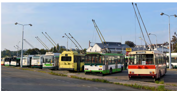
Above: A variety of Škoda trolleybus rear ends. The three 14 Trs on the right show the design differences between the American export, the modernized 14 TrM and the original design.
